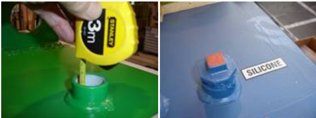
Figure 1. Measure oil level.
